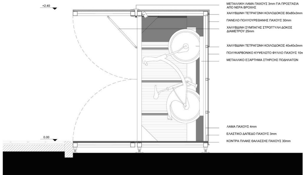
**Figure 5** Longitudinal section of bicycle rental unit
