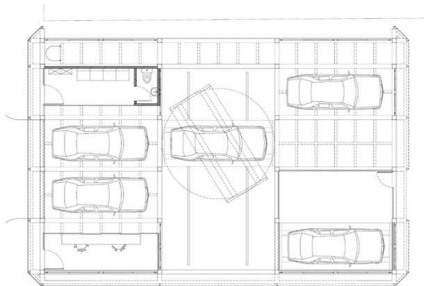
**Figure 3** Ground floor plan of indicative garage types (A2 and B), with a capacity of 12 and 52 cars respectively
